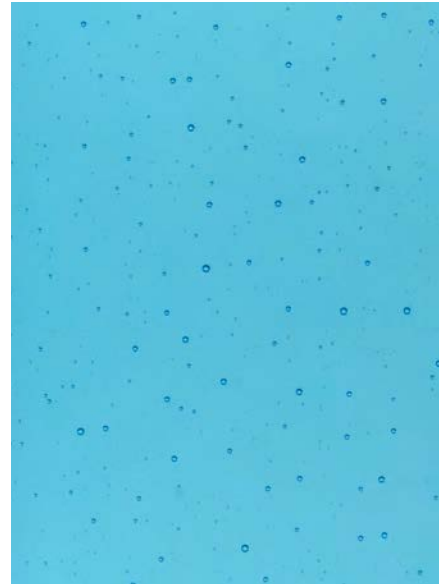
For comparison, same sheet glass lay-up fired without powder to a basic full fuse. Typical champagne bubbles.
